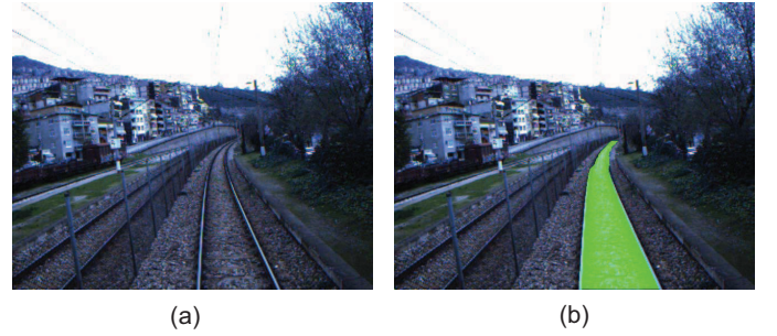
Fig. 8. Examples of railroad track extraction on various scenes: a) Original image b) Result of railroad track extraction
