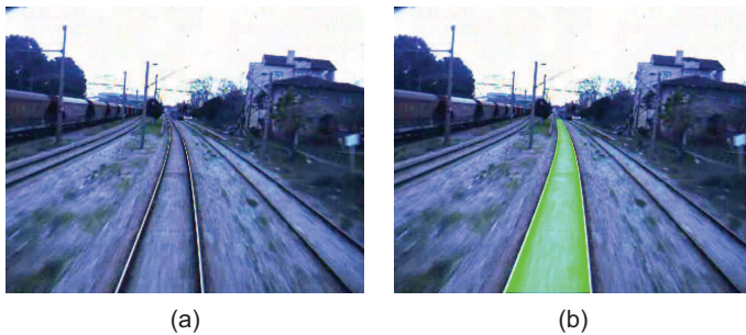
Fig. 11. Examples of railroad track extraction on various scenes: a) Original image b) Result of railroad track extraction
