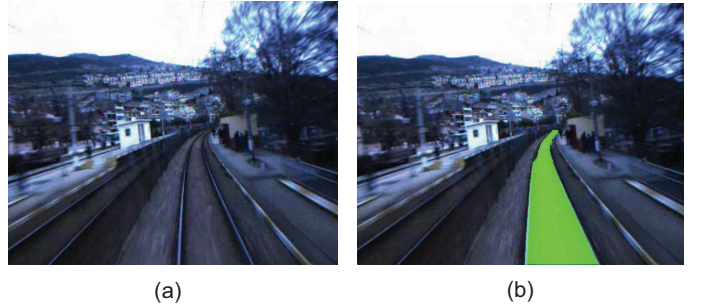
Fig. 9. Examples of railroad track extraction on various scenes: a) Original image b) Result of railroad track extraction
